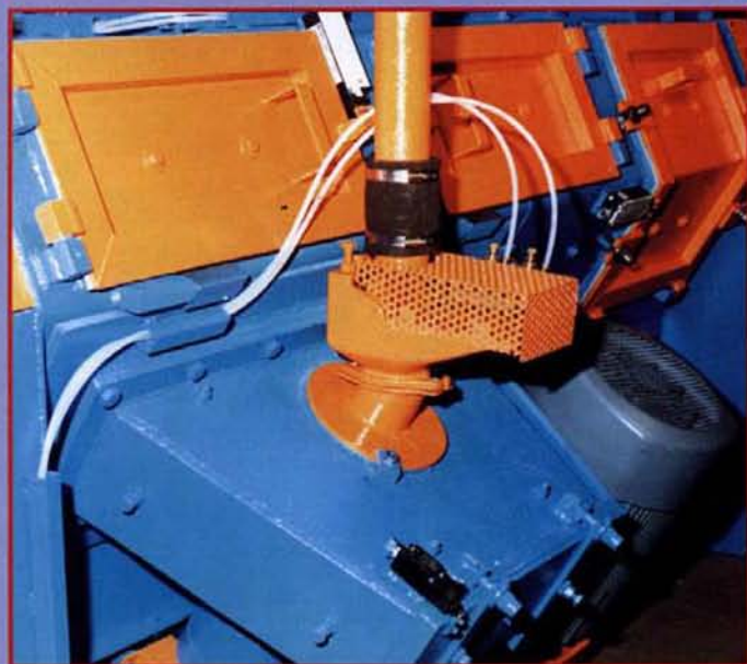
Detail of bottom turbine mounted on hinged rotating frame in order to do an easy maintenance
